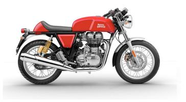
Single Cylinder, 4 stroke, Air cooled
